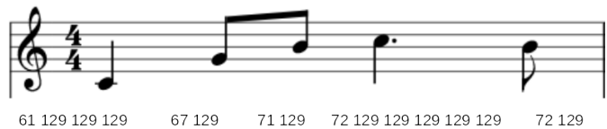
Figure 2: Integer representation of a monophonic melody. Values 0–127 represent MIDI “note on”, 128–“note off”, and 129–“no change”. The first quarter note is represented by four integers where the first denotes the MIDI pitch and the next three indicate that there is no change for the next three semi-quavers.
