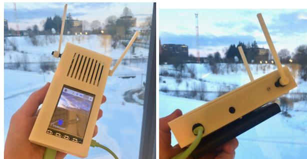
Figure 1: Our prototype interface; the left lever allows user input, and the right lever represents RNN output. A demo can be viewed at <https://youtu.be/0XQ0hRCsbhU>
